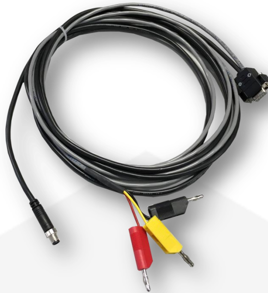
Figure 7: Y Cable CT-I (Red: I_S , Black: I_S return, Yellow: shield)
