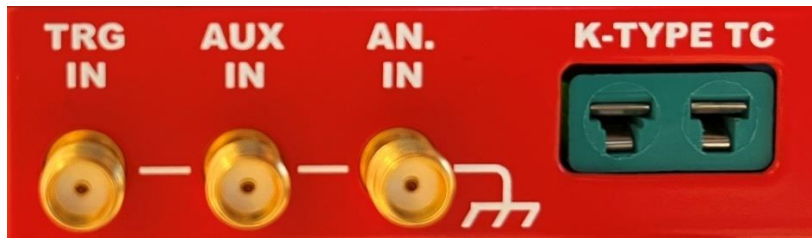
Figure 22: SMA jack input connectors and Type K IEC for thermocouple.
