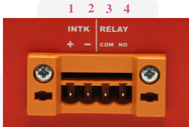
Figure 7: Interlock connector on the unit rear panel
