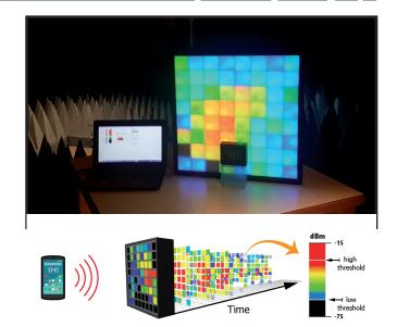
Direct visualization in 3D on PC acquisition of 64 sensors. Setting thresholds in real time.
